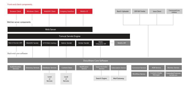
The DocuShare architecture diagram provides a simplified overview of the relationships between the major DocuShare components. DocuShare core software is broken into a series of long-running processes that handle main server tasks, with mid-tier server components handling web requests and generating the UI. The front-end client components provide an HTTP/XML interface that allows many clients to communicate with DocuShare.
