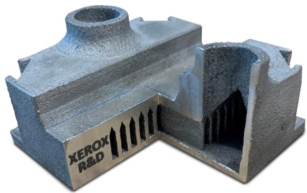
3 Quarter View of the Aluminum 3D Printed CPU Cooler with custom internal channels
