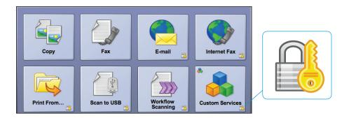
A touch-screen user interface from a Xerox WorkCentre MFP shows how IT administrators can choose to require authentication for specific walk-up features and functions.
