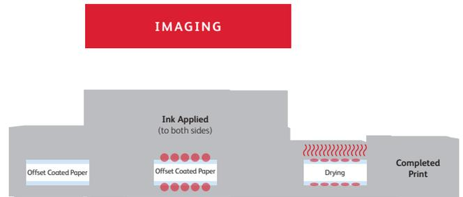
With the Xerox® Trivor® 2400 HF Inkjet Press and Xerox® High Fusion Ink and Xerox® Baltoro™ HF Inkjet Press, there is no need for pretreatment. Both presses use ultra compact drying systems to reduce footprint, drying times, energy use, maintenance and supplies.
