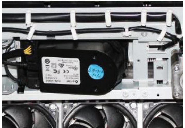
The X-Rite® Inline Spectrophotometer automates the collection of XRGB data for calibration and profiling.
