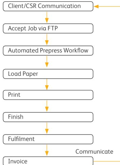
Book sizes and shapes vary. Covers and body content can come from multiple sources. All this adds up to more prepress time being spent preparing the files for print. Prepress automation, as outlined in the diagrams above, can eliminate hours from your book production process.
