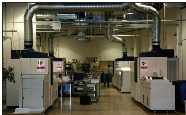
Some of the six Xerox iGen3® 110 Digital Production Presses at QuantumDigital, which contribute to the company’s environmental sustainability, according to the company’s Chief Operating Officer Freddie Baird.
